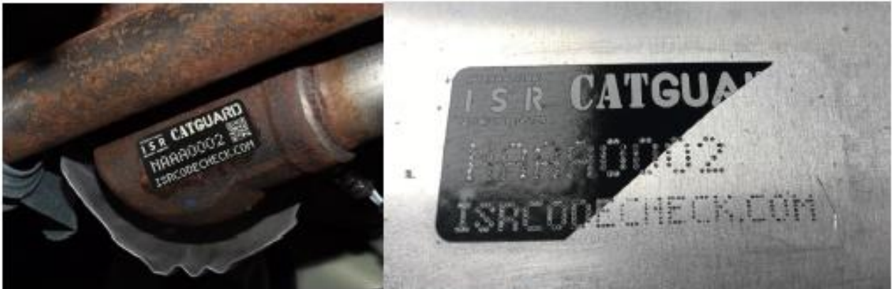
The above photos are sample images of catalytic converter labels produced by RETAINAGROUP – IAATI does not endorse specific products, the above examples are for illustration purposes only.
