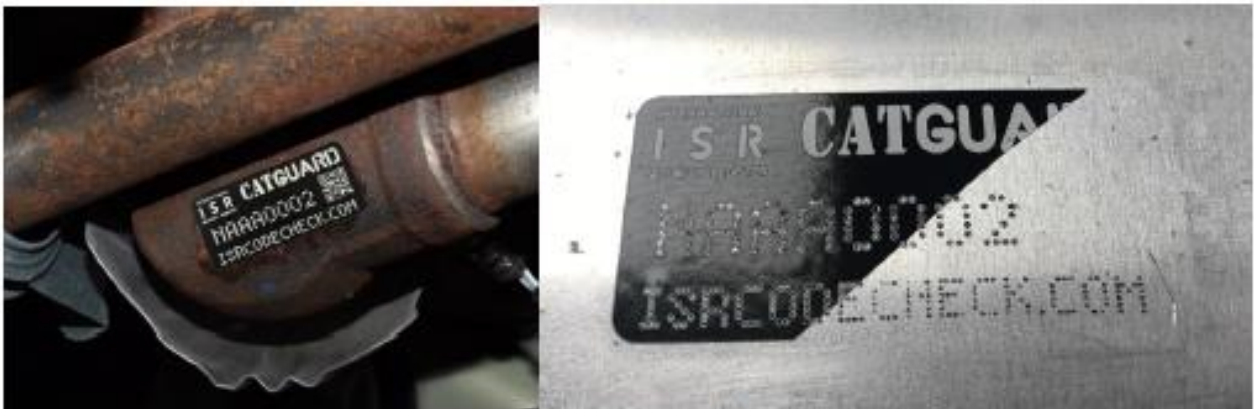
The above photos are sample images of catalytic converter labels produced by RETAINAGROUP – IAATI does not endorse specific products, the above examples are for illustration purposes only.
