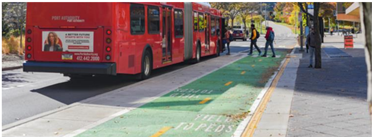
FIGURE 15: ELEVATED BUS STOP EXAMPLE
