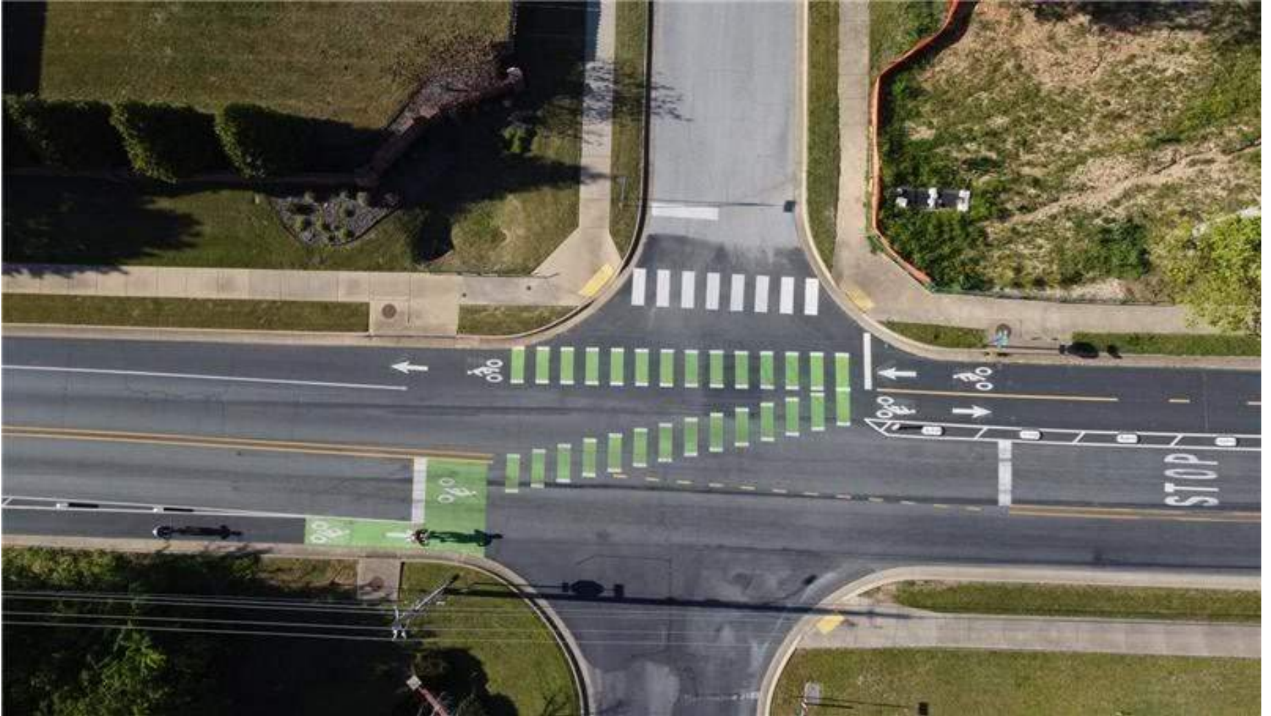
Figure 31: Transition from two-way cycle track to buffered bike lanes in Bentonville, AR.
