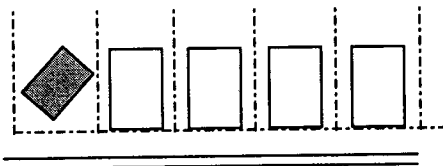
Inappropriate building orientation
