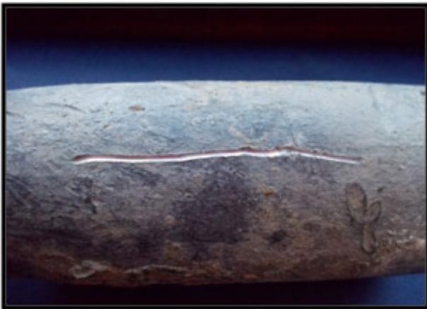
Lead service lines are generally a dull gray color and are very soft. You can identify them easily by carefully scratching with a key. If the pipe is made of lead, the area you've scratched will turn a bright silver color. Do not use a knife or other sharp instrument and take care not to puncture a hole in the pipe.
