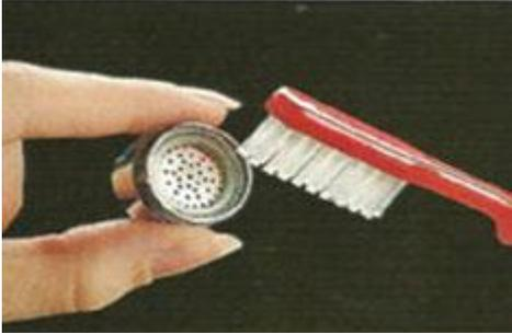
Step 3. Rinse the pieces with water and brush off the debris. For deposits that are difficult to remove, soak the parts in water for a few minutes and scrub with a toothbrush. Backwashing aerator components is also an effective cleaning method for many aerator types. Hold the removed aerator upside down under flowing water to backwash screens and mesh filters.
