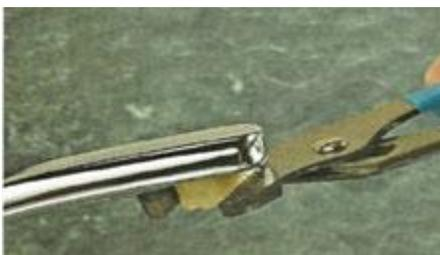
Step 1. Remove the aerator by twisting off with hands or pliers.
